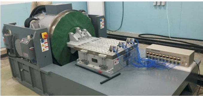
Vibration Test Equipment
